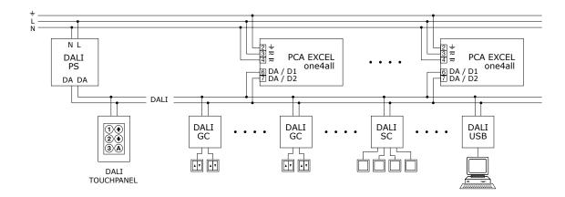
Wiring diagram for operating with push buttons or touch panel
