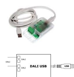
The Dali network is controlled by the computer via the Dali USB interface module. Specially developed software enables the entire control function of the lighting system to be programmed.
