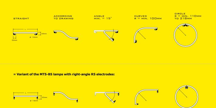
These lamps have the same properties as MT5-B5 lamps, but with their right-angle electrodes they can be integrated perfectly into a ceiling or wall. This means that they are also extremely well suited for use in wall lighting.
